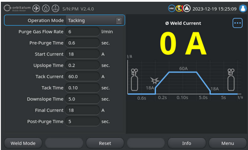
Illustration: Manual programming, tack welding operating mode
