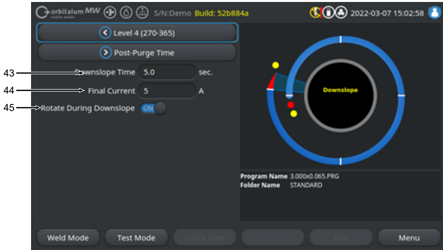
Illustration: "Downslope" section of the welding procedure
