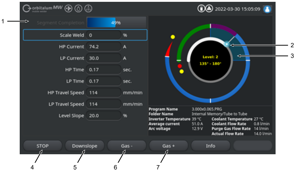
Illustration: View during active welding process
